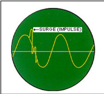
Surges on power systems -- also known as transients -- result from energy being released into the system. In low-voltage AC power circuits, surges have two basic origins: lightning or switching events.
